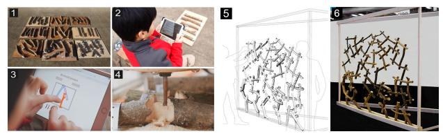
Figure 1: Workflow overview: 1.fix branches on plates 2.scan the plates and upload the model 3. play the game with scanned branches 4.fabricate joineries by a CNC router 5. The layout of a screen wall designed for South by South West (SXSW). 6. An assembled screen wall.
