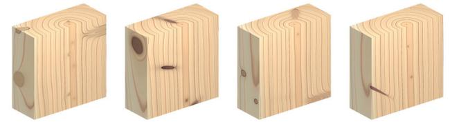
Fig. 16. Rendered images of same portion of a tree, with randomized parameters and knot skeletons (same wood color map).
