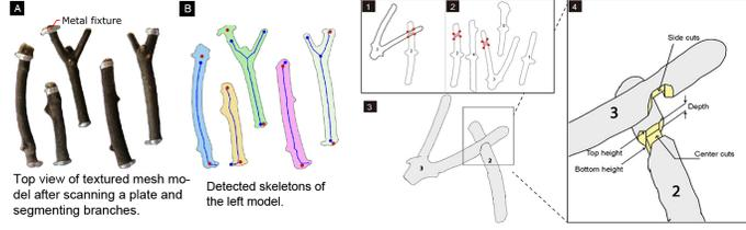
**Figure 2:** Left: A and B show an interface of branch importer. Right: diagram of our joints. 1. A layout design 2. Branches on a plate with milling paths in red 3. An assembled pair of branches 4. A close-up joint geometry.
