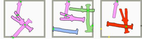
**Figure 4:** Left: valid group with two target points connected. Middle: valid but non-optimal because there is more than one group. Right: invalid due to Islanded situation.
