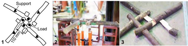
**Figure 20: Flexural test. 1,2: Experimental setup. 3: Failure mode.**
