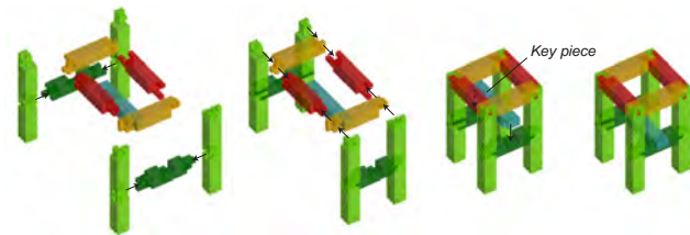
Figure 23. Interlocking stool assembly with eleven pieces connected by four unique 3-timber joints and six unique two-timber T-joints.
