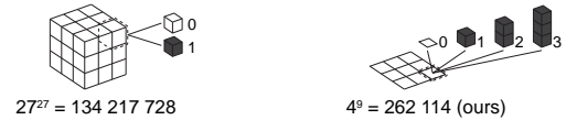
Figure 11. For a two-timber joint in 3 \times 3 \times 3 resolution, the number of possibilities for a voxelized cube (left) compared to the height field representation (right).
