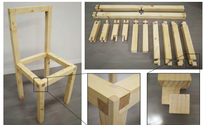
Figure 20. Chair fabricated from 12 timbers connected by nine nail-free and glue-free joints.
